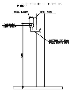
DETALHE DO GUARDA-CORPO SEM ESCALA
