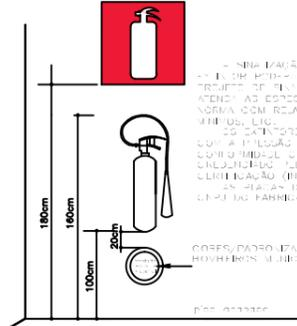
DETALHE TÍPICO DO EXTINTORES SEM ESCALA
