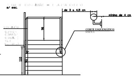
DETALHE DO GUARDA-CORPO SEM ESCALA
